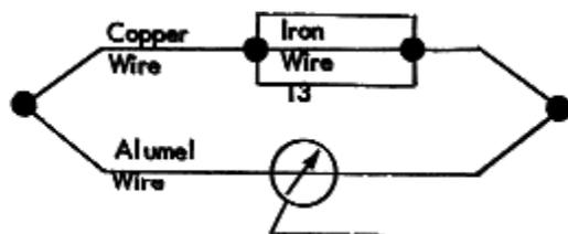
A consequence of this law is that if one junction of two dissimilar metals is maintained at a temperature  $T_1$  and the other junction is at  $T_2$ , the thermal EMF developed at the junction will not be affected by the temperature of the lead wires even though a
