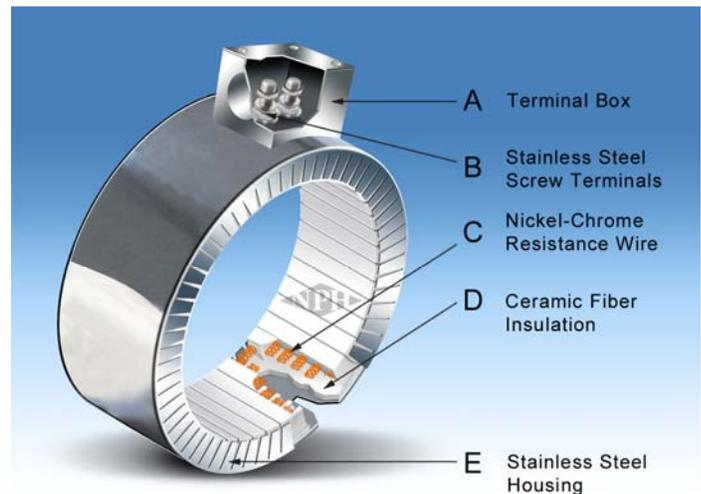
**Ceramic Band/Knuckle Heater-Construction Components**
