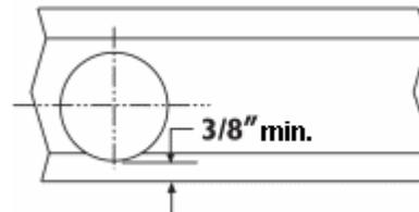
When a hole is offset to one side of a heater there must be a minimum of 3/8" clearance from edge of hole to edge of heater on one side of the hole
