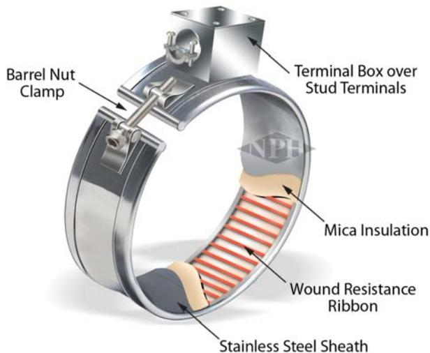
**Mica Band Heaters-Construction Components**
